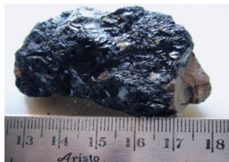
Fig 2: A picture of coltan admixed with feldspar and mica collected from the mine dump of abandoned mica northeast of parlappalli, podalakur Mandal.
