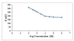
Fig.1: Profile of the Potential in mV/-Log CB Molar Concentration Using Sensor I CB-AR/DBP/Carbon [1×10-4 M -1×10-2 M].
