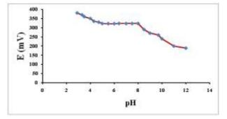
Fig. 3: Effect of pH on the Response of Sensor I CB-AR/DBP/Carbon Using 1.00×10-3 M [Working pH Range: 5-8].
