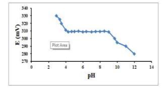
Fig. 4: Effect of pH on the Response of Sensor II CB-PTA/DBP/Carbon Using 1.00×10-3 M [Working pH Range: 4-9].
