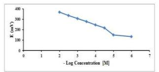
Fig.2: Profile of the Potential in mV/-Log CB Molar Concentration Using Sensor II CB-PTA/DBP/Carbon [5×10-5 M -1×10-2 M].
